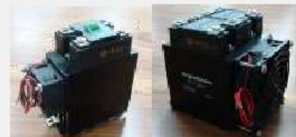
Value added assembly with standard relay / heatsink / Fan
